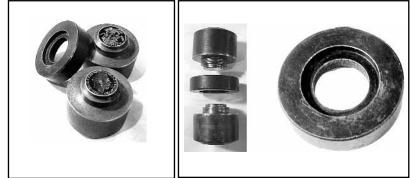
Pictured above at left is the obverse die of a gold sovereign, the reverse die and the collar, or die with the edge, in this case, reeded. In center are the three dies in position. At right is the collar.
